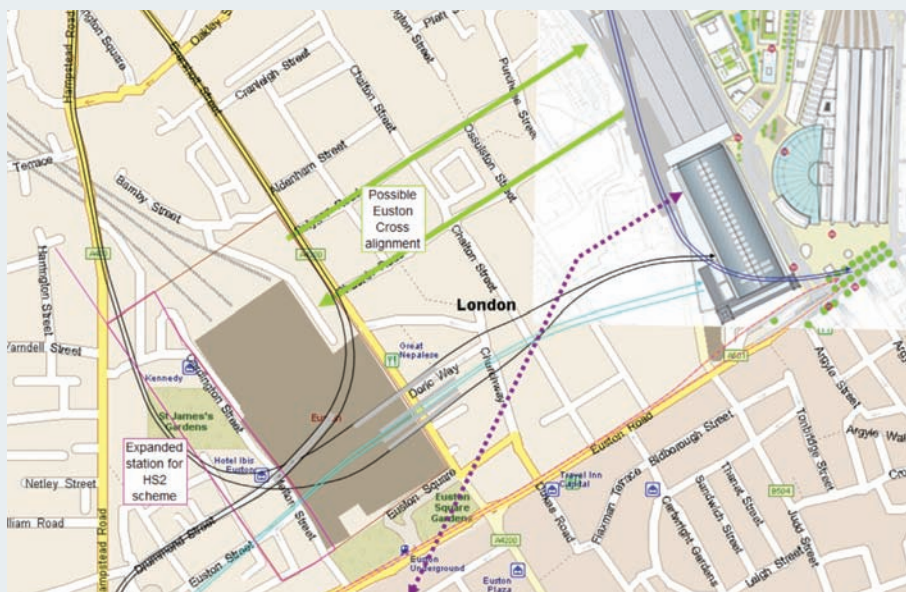
Euston Cross: possible alignment of passenger concourses shown in green (500 metre length) north of potential Crossrail 2 route, shown by dotted line running south west to north east. Bored rail tunnels could be alongside concourses. Pink area is current HS2 expansion proposal for Euston terminus. Other rail alignments are shown.
